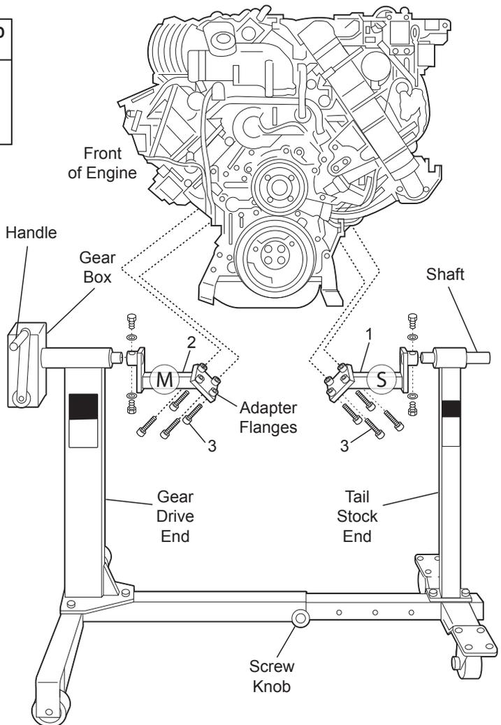
4. Lower the engine with engine stand attached very slowly to the ground so all four wheels of the engine stand are firmly planted on the ground before disconnecting the shop crane from the engine.
